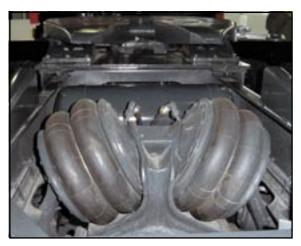
The air springs can be mounted either individually or in panels (where the requested number of air springs is connected), depending on the weight of the vehicle (device). The rubberized-fabric wall of the body must not come into contact with sharp or hot objects (iron scale, edges, exhausts, etc.)
