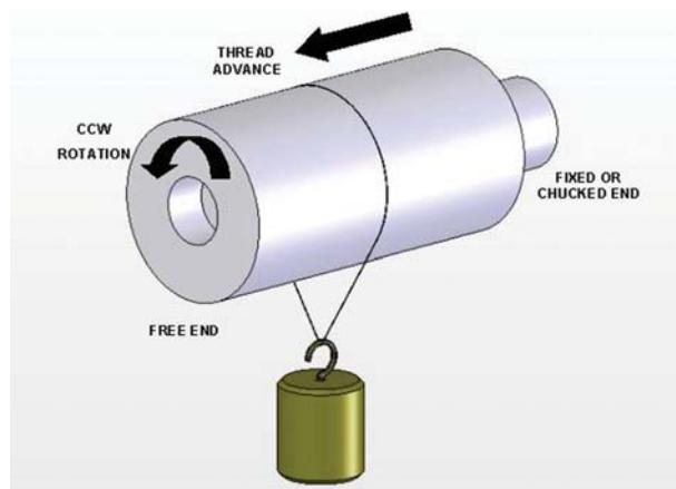
Figure 3: Counter-Clockwise Lead
