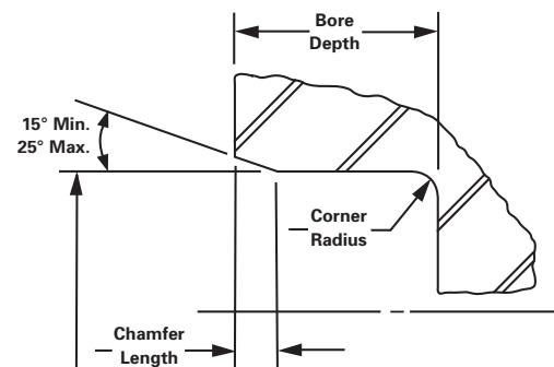
**Figure 8: Housing Bore Dimensions**
