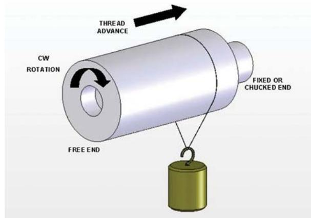
Figure 4: Counter-Clockwise Lead
