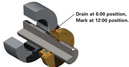
**Figure 15: Drain Port Positioning**
