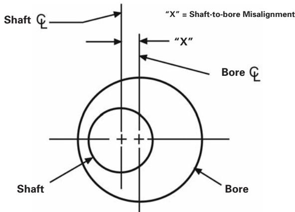
**Figure 5: Shaft-to-bore Misalignment**
