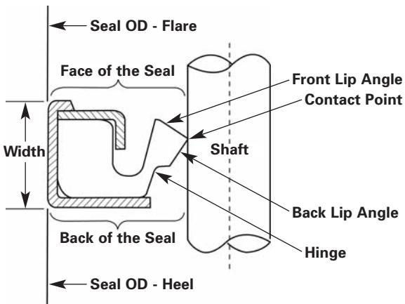
**Assembled Seal:** Seal made up of a group of parts, including sealing surface(s), provisions for initial loading and a secondary sealing mechanism to accommodate radial movement required for installation and operation.
